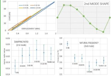
The vibration response is highly sensitive to the tendon cut and it can be used for damage detection.
